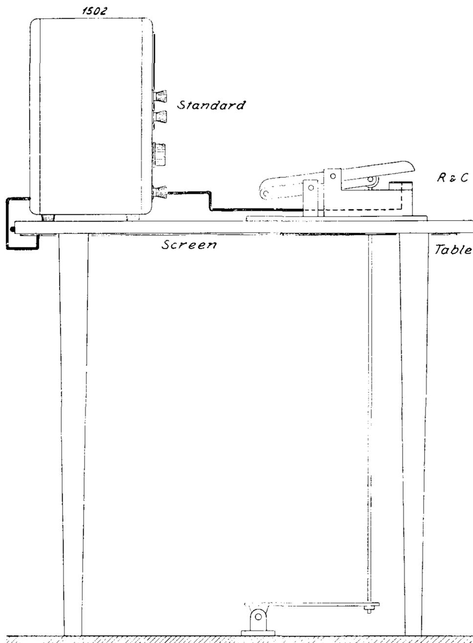
*Fig. 2. Set-up foot-operated contact on screened table.*
