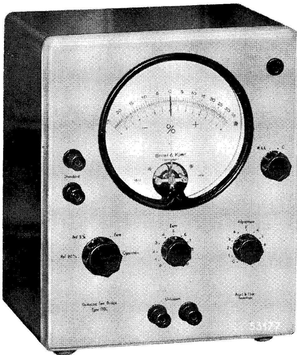
*Fig. 1. Photograph of Deviation Test Bridge type 1502.*
