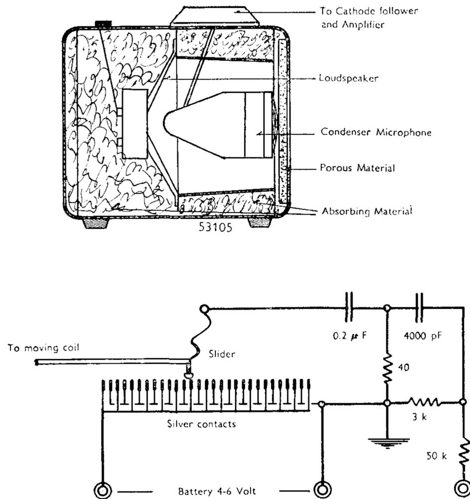
Fig. 4. Cross-section of sound source with flat frequency characteristic and high internal acoustic impedance. Below: principle of the contact arrangement for counting the total length of the frequency curve.
