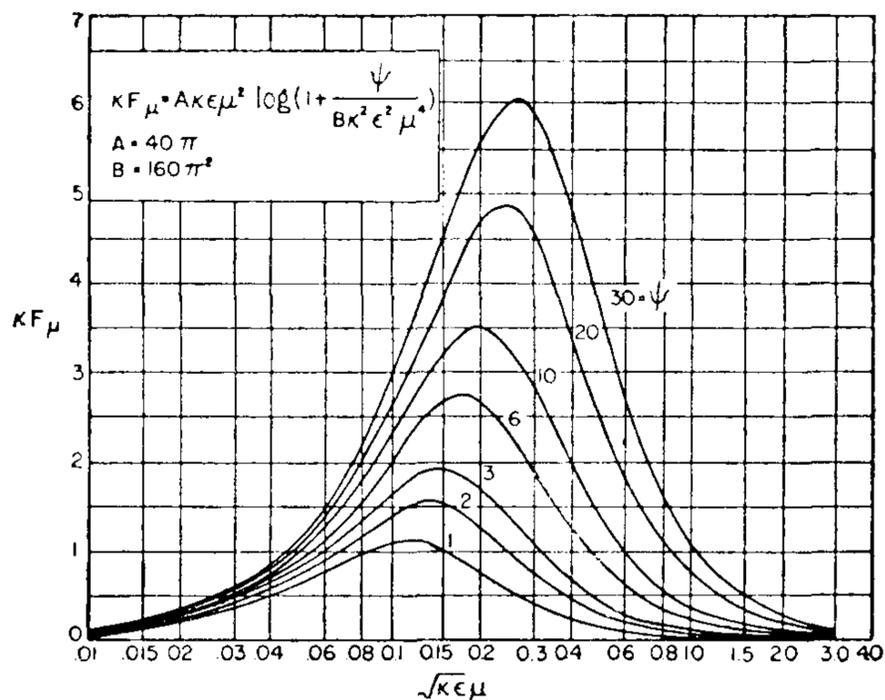
Fig. 10. Generalized plot of frequency irregularity functions from approximate theory from Bolt and Roop.
