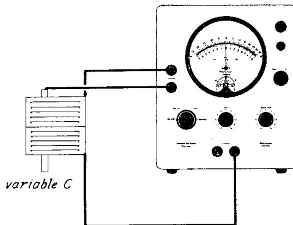
*Fig. 6. Matching of variable condensers.*
