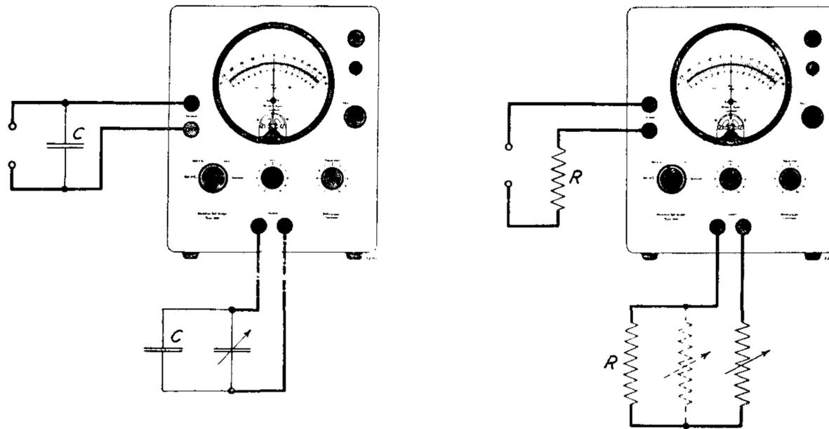
*Fig. 8. Direct reading measurements of capacity and resistance values.*
