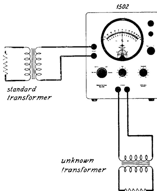
*Fig. 7. Production testing of transformers.*
