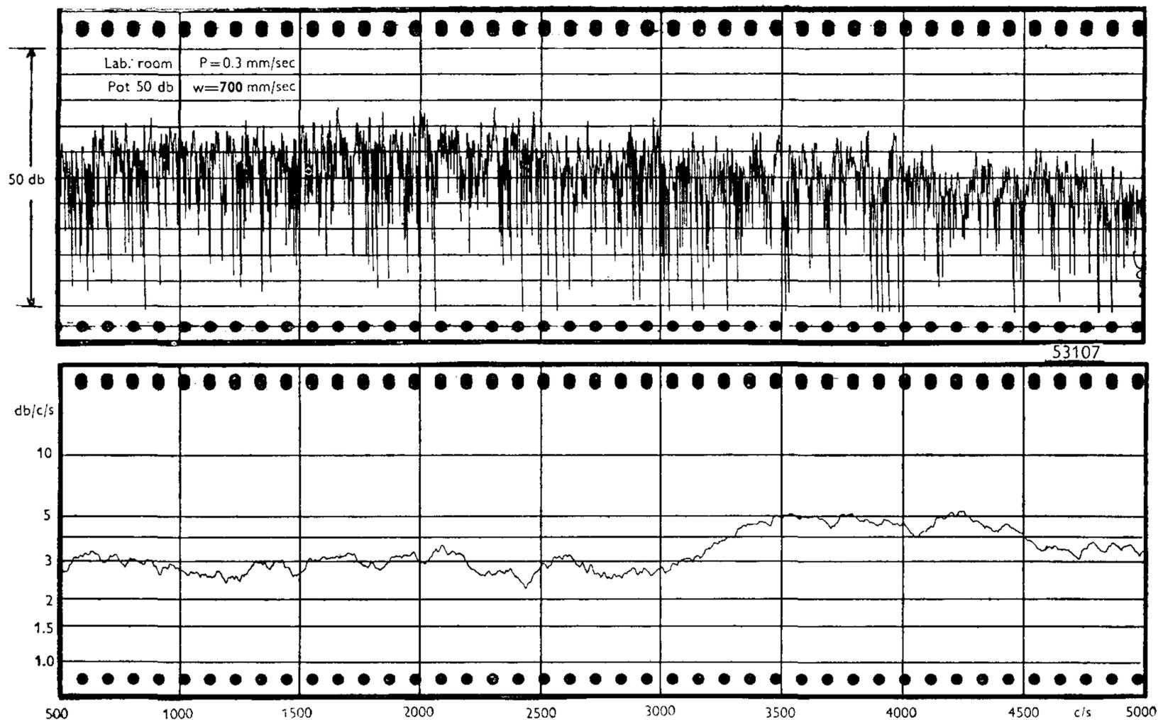
Fig. 7. Frequency Response Curve and curve of "Frequency Irregularities" for a laboratory, recorded with the set-up of fig. 6.
