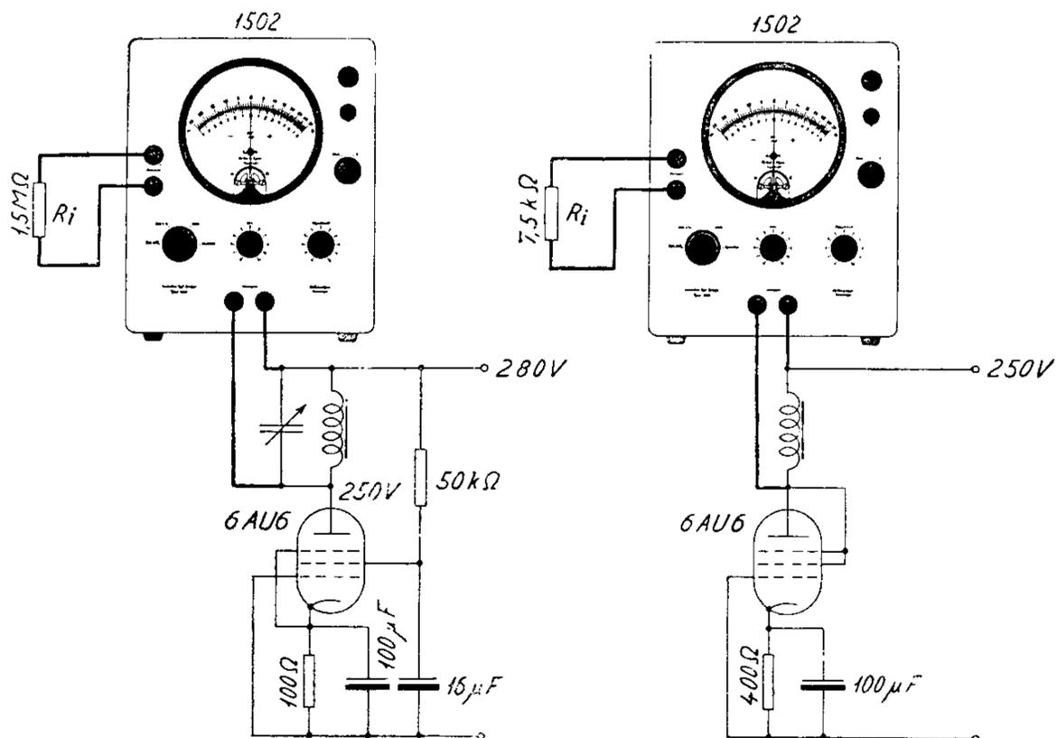
Fig. 10. Measuring internal resistance of 6AU6 tube connected respectively as pentode and triode.
