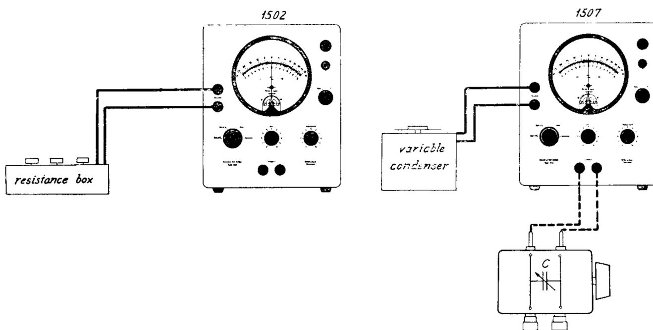
Fig. 5. Resistance box connected to 1502 and variable condenser to 1507.
