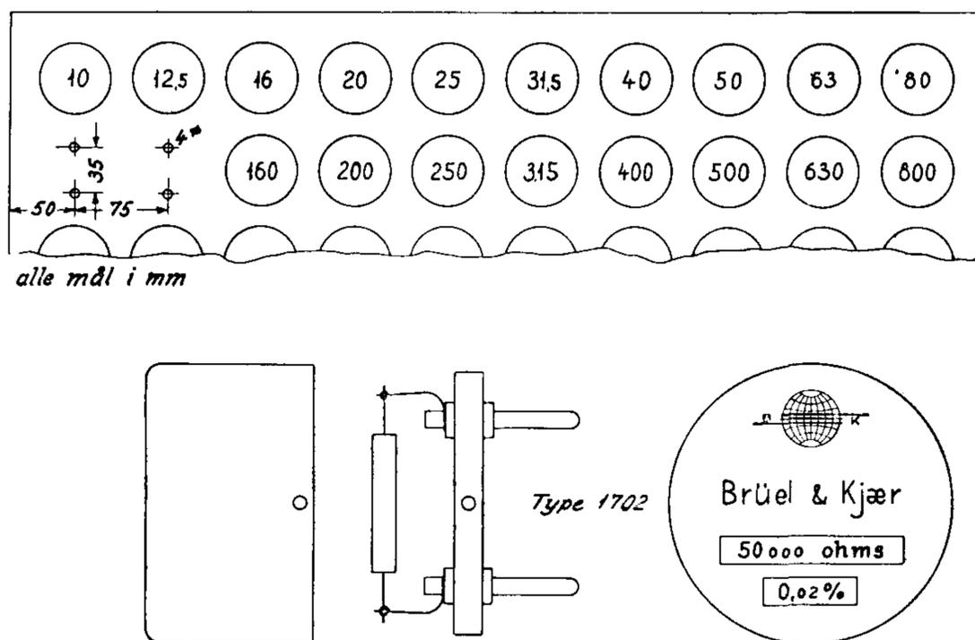
Fig. 4. Practical arrangement for standard resistance values. The standard resistances are placed in our Standard Box type 1702.
