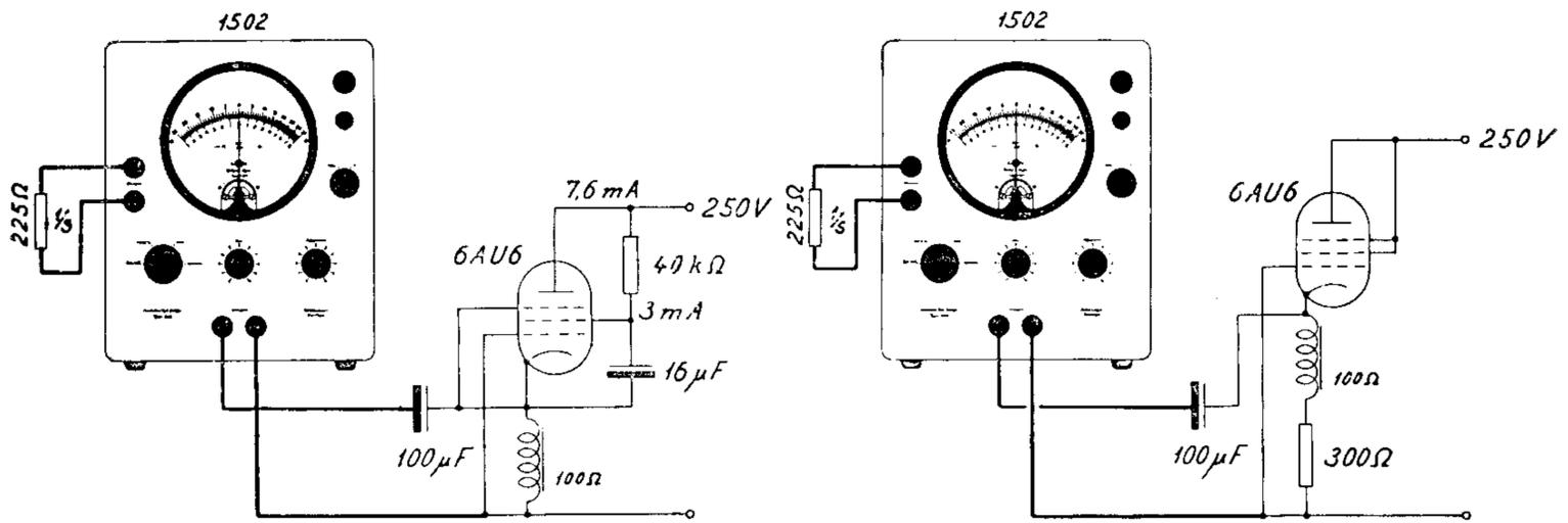
Fig. 9. Measuring transconductance of 6AU6 tube connected respectively as pentode and triode.
