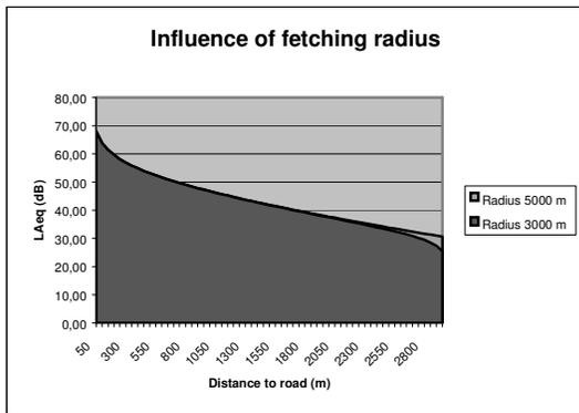
Fig. 04: Levels for 3000 m or 5000 m fetching radius
