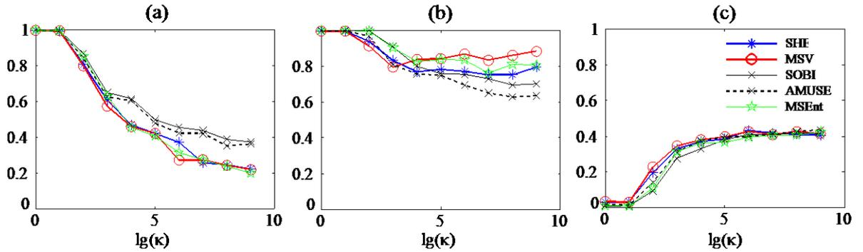
Figure 5: Comparison of separation results for increasing condition  $\kappa$  numbers with  $F_s/\zeta\omega = 10^{-2}$ , SNR = 20dB, and  $m = n = n_e = 4$ : a) correlation coefficient, b) MAC, c) relative “cross-talk” error.
