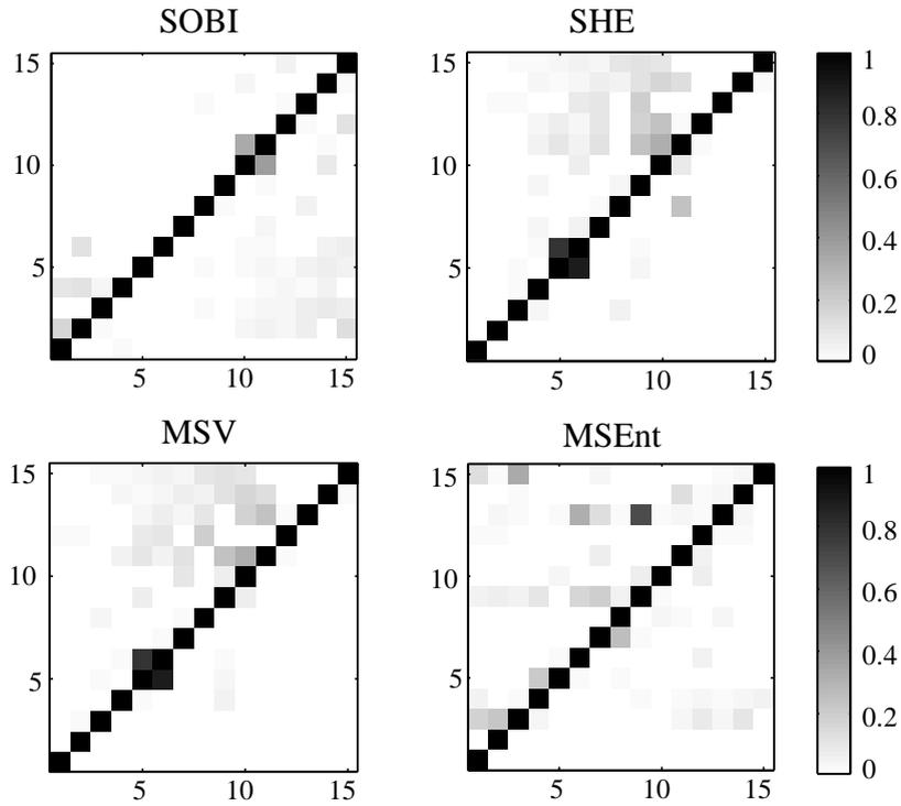
Figure 10: Matrices of values  $e_{ij} = |\hat{\phi}^i \phi_j| / |\hat{\phi}^i \phi_i|$  reflecting the closeness of the separation matrix to the actual inverse of the modal matrix ( $e_{ij}$  are ideally the elements of the identify matrix).
