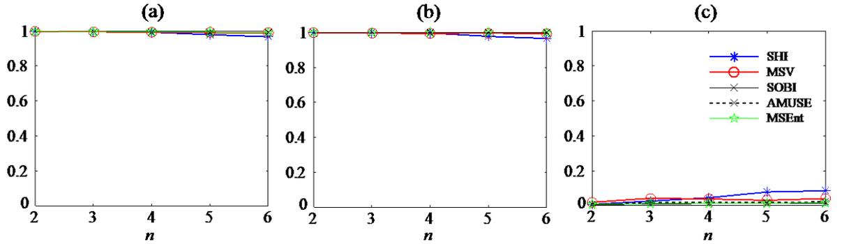
Figure 6: Comparison of separation results for increasing numbers of degrees of freedom  $n$  with  $F_s/\zeta\omega = 10^{-2}$ , SNR = 20dB, and  $m = n = n_e = 4$ : a) correlation coefficient, b) MAC, c) relative “cross-talk” error.
