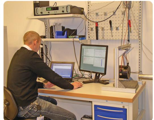
The testing setup on the front side of the seal mounting test plate
