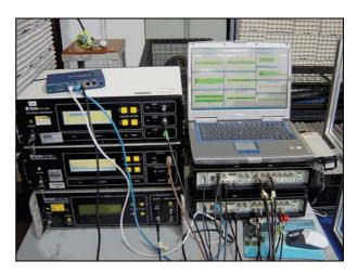
The software used includes PULSE FFT & CPB Analysis Type 7700 and Time Capture Type 7705.
