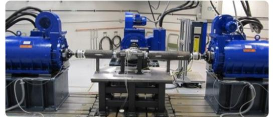
The TE and Mini-TE test stands both use a PULSE front-end as the primary data acquisition system (analysis frequency range of 0 – 25.6 kHz) and a Brüel & Kjær Optical Tachometer. The new test stands also include a PULSE Data Acquisition System – 30-channels with Analysis Frequency Range of 0 – 25.6 kHz and 12 Aux. Channel Tracking.
