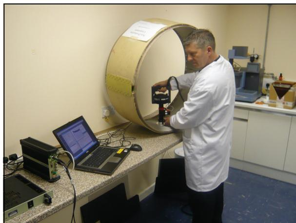
GKN has carried out pure tone tests at a user-specified frequency and broadband noise tests, up to 155 dB overall sound pressure level, measured at the face-sheet, on small scale, flat acoustic material specimens, as well as full scale panels. This is within a design down selection exercise, whereby a comparative analysis of these measurements with the prediction of a proprietary normal impedance prediction model, has also been performed.
