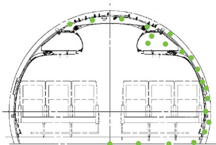
Distribution of multi-field microphones in the cavities between the cabin and the fuselage
