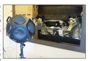
five and thirty measurements can be made and the test data compared during post-process analysis. The NVH parameters of the test object are either defined by Carcoustics, based on its great experience, or specified by the customer in relation to NVH targets for a complete vehicle or component.
