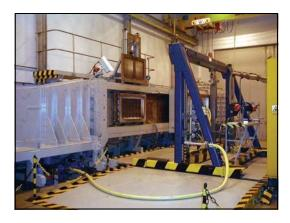
ronment similar to that seen on an aircraft during flight. The specimen is held on a moveable loading frame and is usually built up so that the specimen forms the closing wall to the working section. The cross-section area can be reduced by inserting sleeves within the duct to required depths".
