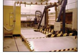
some test requirements have been fulfilled with narrow band noise levels of  $170\,\mathrm{dB}$  RMS at  $40\,\mathrm{Hz}-a$  unique capability for this facility. The noise generator, essentially a reciprocating poppet valve, can produce controlled noise in the frequency range between  $30\,\mathrm{Hz}$  and  $500\,\mathrm{Hz}$ . at levels of up to  $175\,\mathrm{dB}-l$  louder than the near-field noise levels of the jet efflux of a Eurofighter Typhoon on full reheat.
