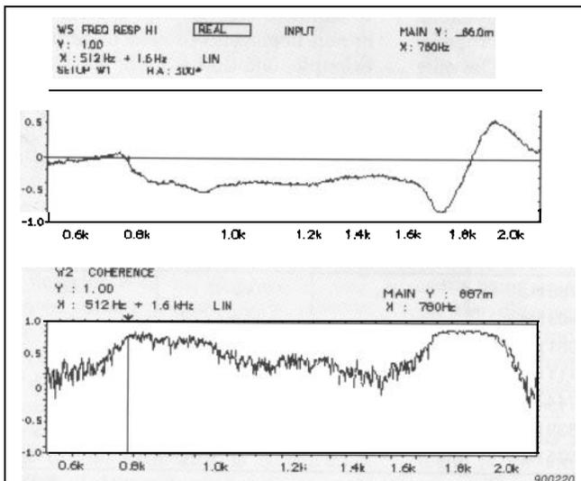
Fig. 6. A typical FRF measurement. For measurement point 24, the real part of the FRF and the coherence are shown
