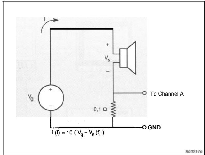
Fig. 4. The 0,1Ω resistor is used to measure the current through the loudspeaker. This allows the excitation channel to be calibrated in terms of force, since the force is proportional to the current
