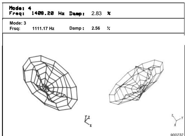
Fig. 11. Example of a stiffness modification near the surround to simulate a change in material. Note the upward shift in modal frequencies
