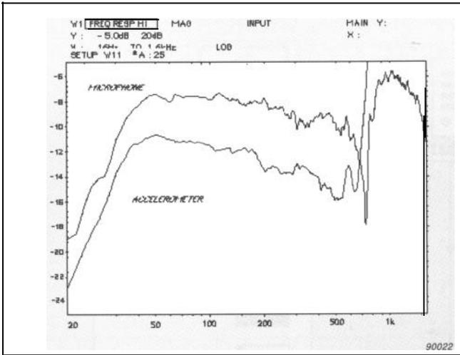
Fig. 3. In the piston range of operation, the near field response is proportional to acceleration. A comparison of the two clearly reveals when the diaphragm no longer behaves as a rigid structure
