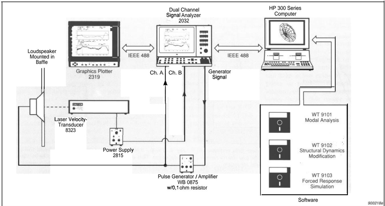
Fig. 1. Test configuration
