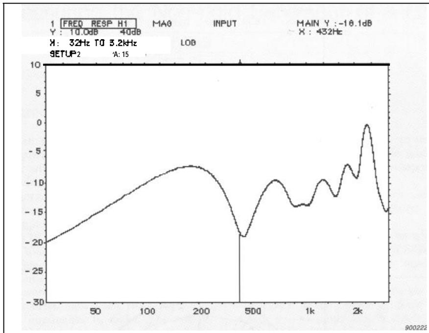
Fig. 12. A measurement showing the free field response of the driver. Structural modes contribute to the variations in the response beyond the rigid piston range of operation
