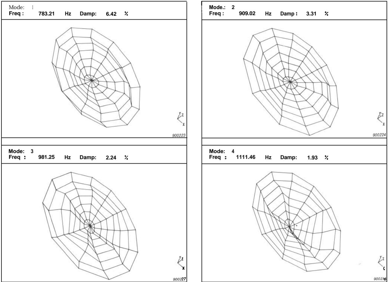
**Fig. 8. Plots of the mode shapes 1, 2, 3, and 4. For each mode shape, the modal frequency and damping are listed above the structure**
