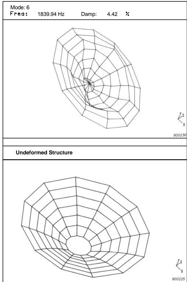
Fig. 9. Plots of the mode shapes 5, 6, 7 and the undeformed diaphragm.
