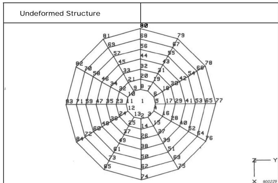
Fig. 5. Measurements were performed at 73 different points around the diaphragm. No measurements were made at the points numbered from 74 to 85. These points represent the driver frame and are used as a reference for the displacement
