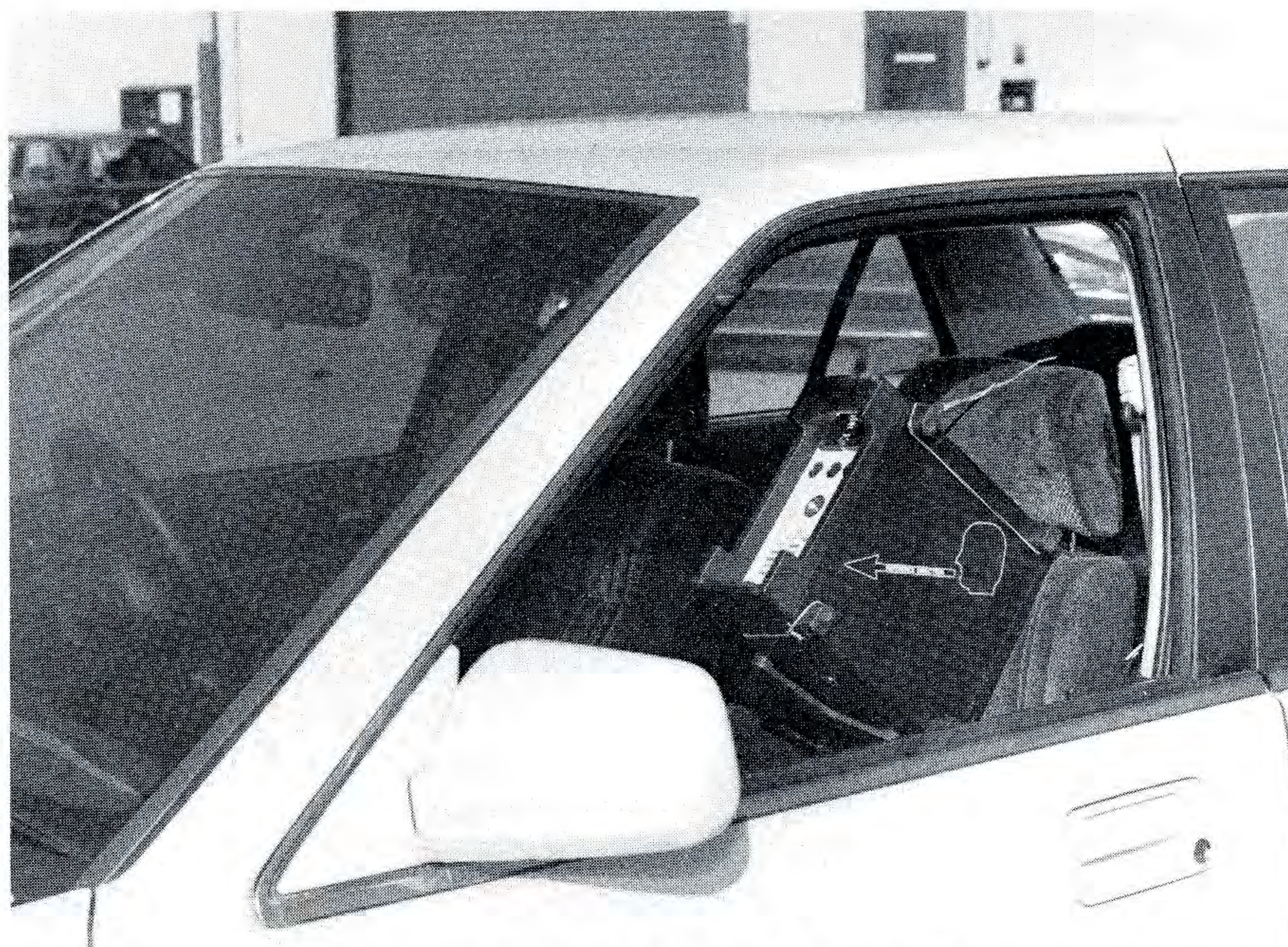
Fig. 6. The transmitter (Type 4225) of the Speech Transmission Meter placed at the front passenger seat
