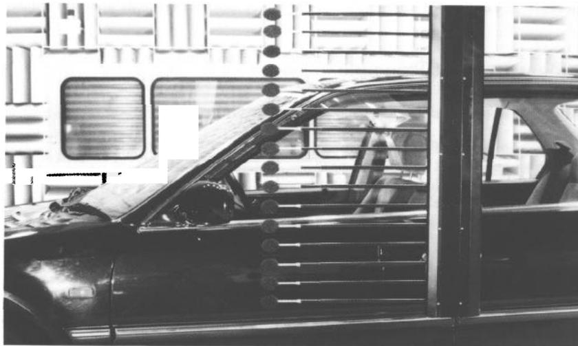
Below, the interior of Honda's low noise wind tunnel. Above, the STSF scan array in use in the wind tunnel
