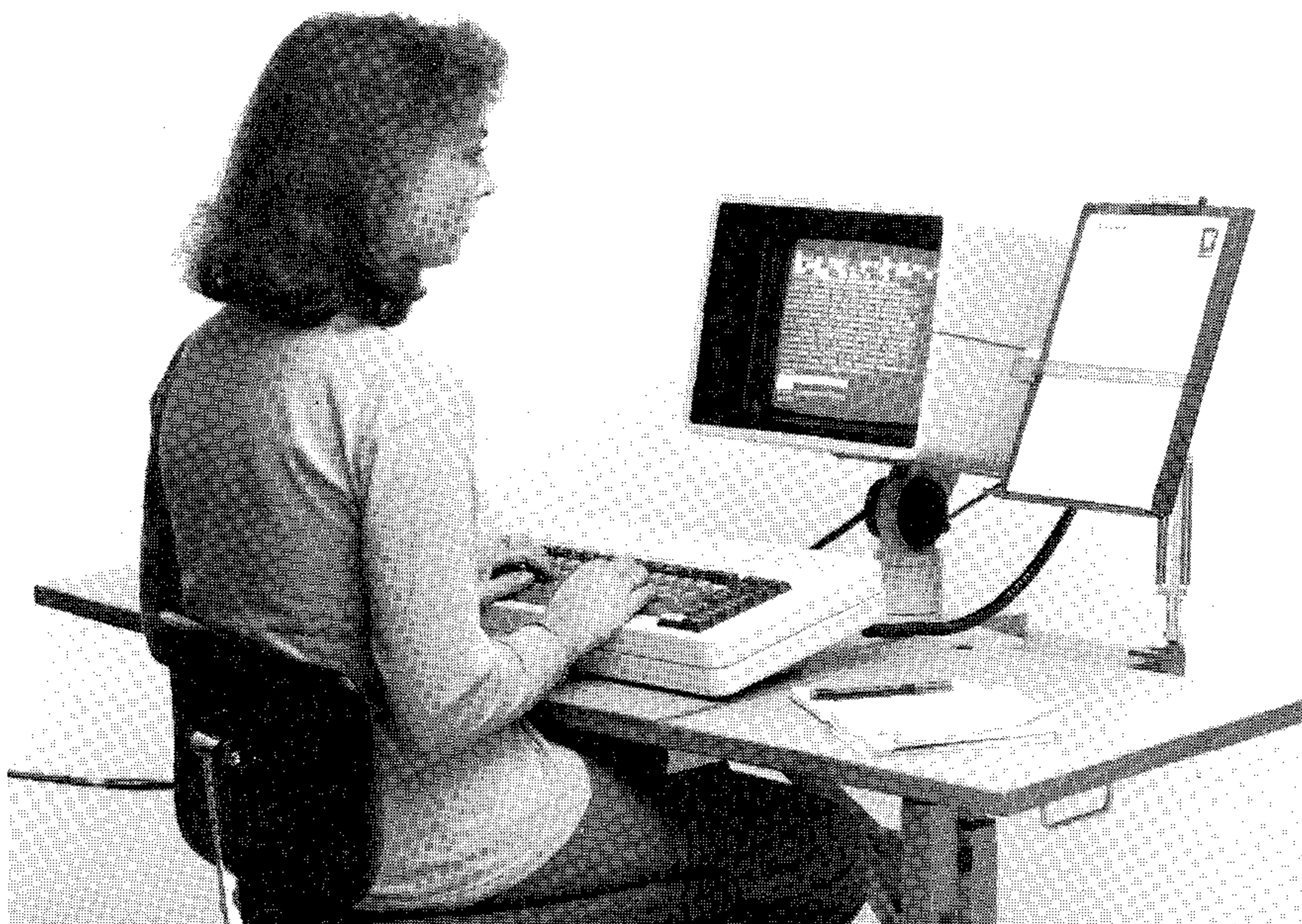
Fig. 2. The three visual tasks at a workplace with a terminal: the screen, the keyboard and the document. But what type of lighting should be installed so that these three tasks are performed under optimal conditions?
