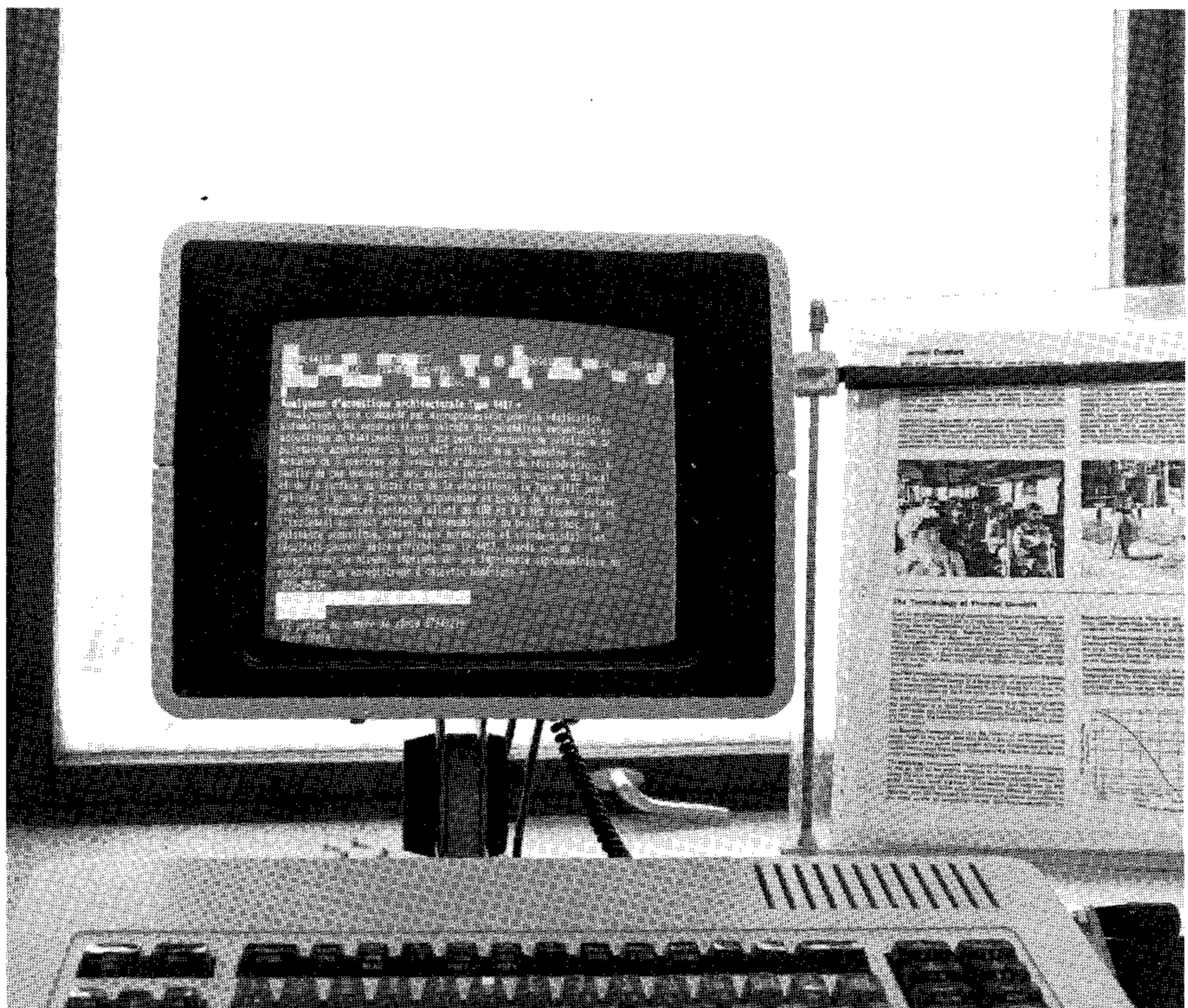
Fig. 8. The disability glare effect from a window in the visual field of an operator.
