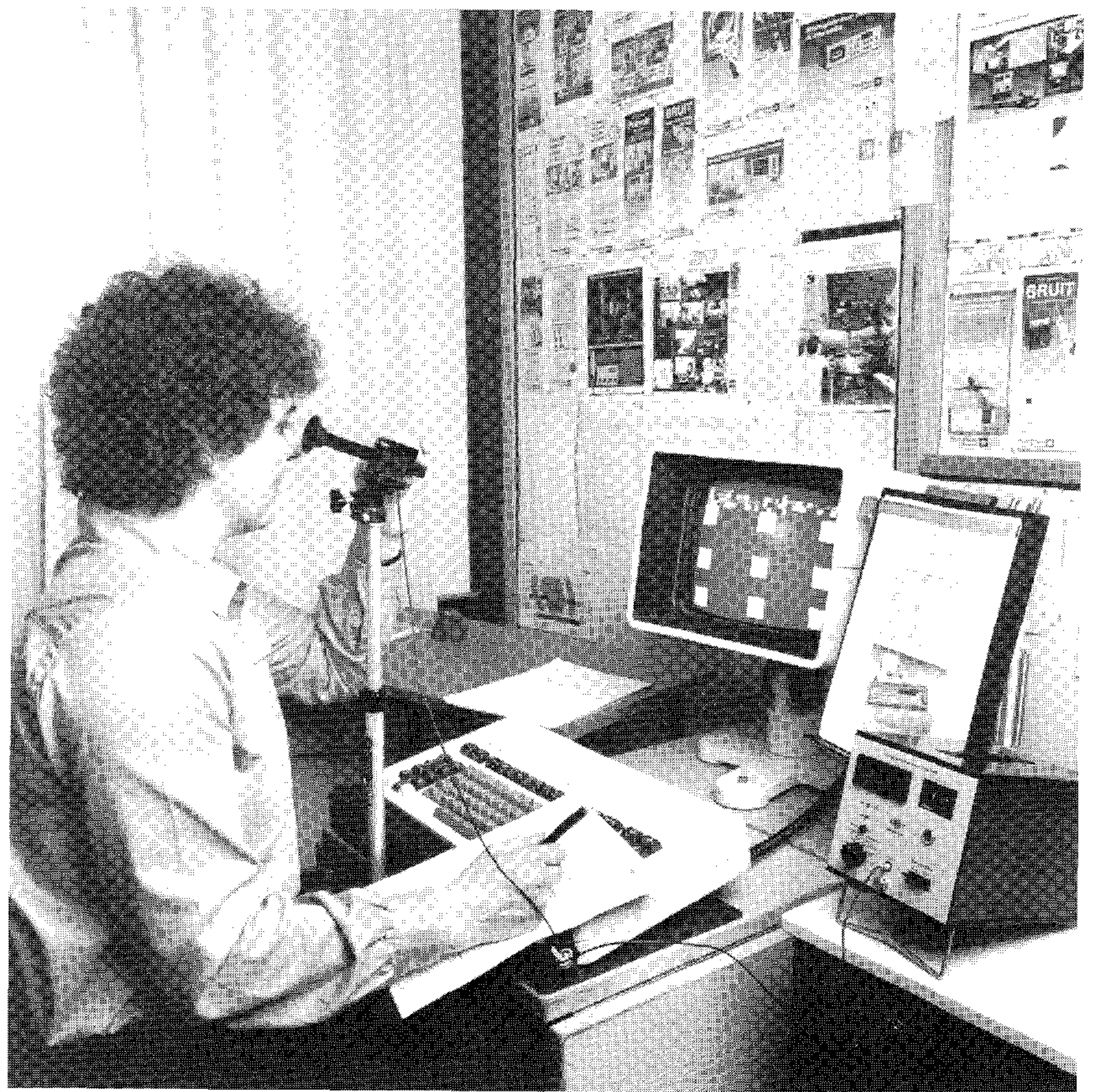
Fig. 11. The instrument memorises the two luminances and gives the value of the contrast. The measuring cell, which incorporates a normalised CIE filter and a narrow acceptance angle, is installed on a sighting mount at the position of the operator's eye and simply pointed towards one of the areas on the screen
