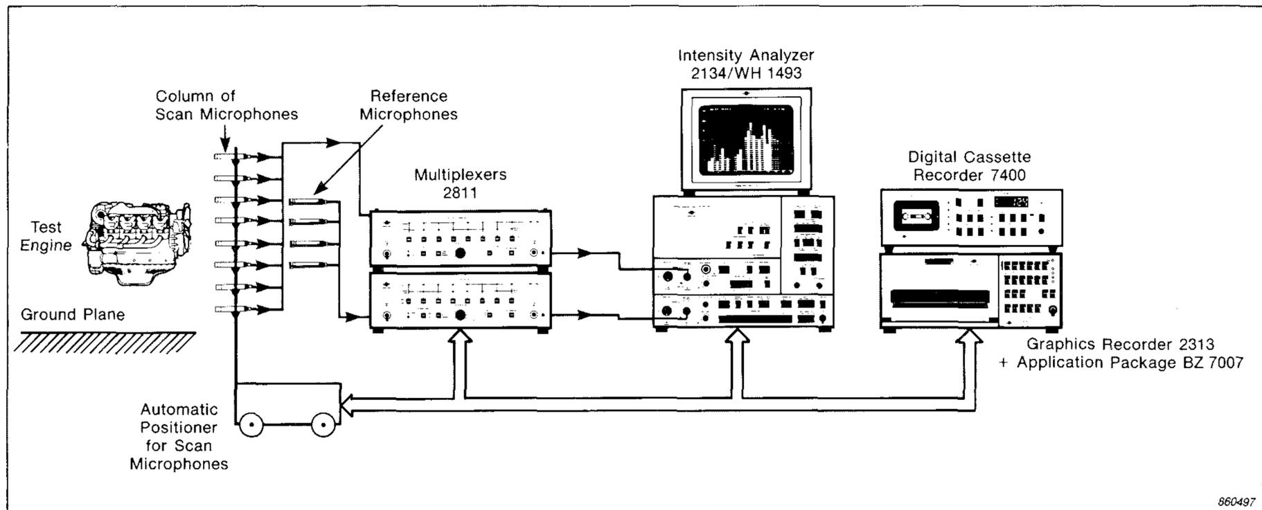
Fig. 1. Instrumentation for STSF
