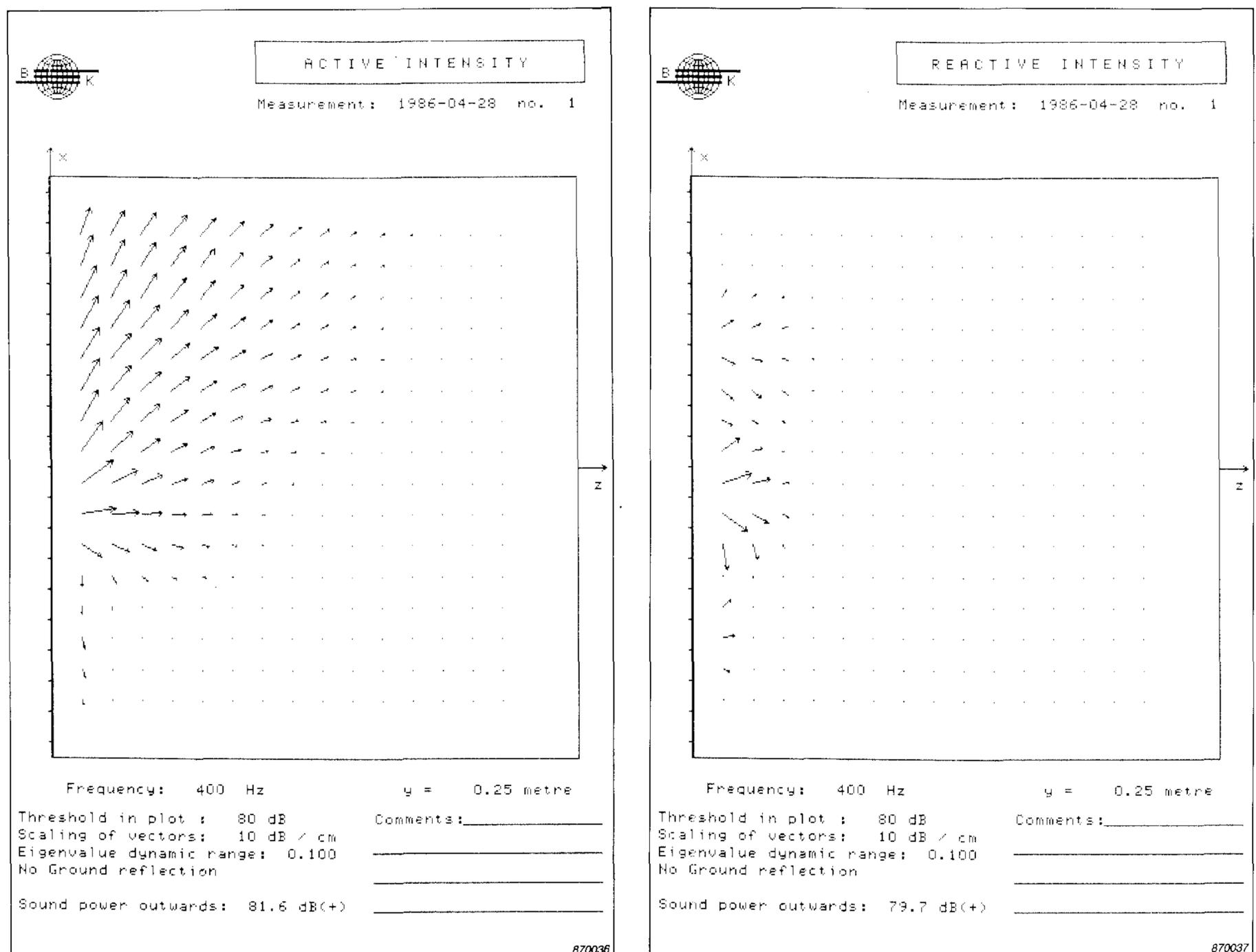
Fig. 10. Plots of intensity vectors in the plane  $y = 0,25$  m for the 400 Hz  $1/3$ -octave band.
