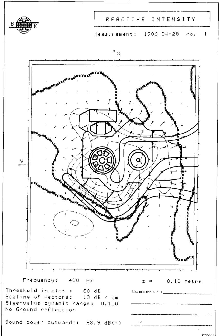
Fig. 12. Combined contour/vector plots of intensity in the plane  $z = 0,1\text{ m}$  for the  $400\text{ Hz}$   $1/3$ -octave band
