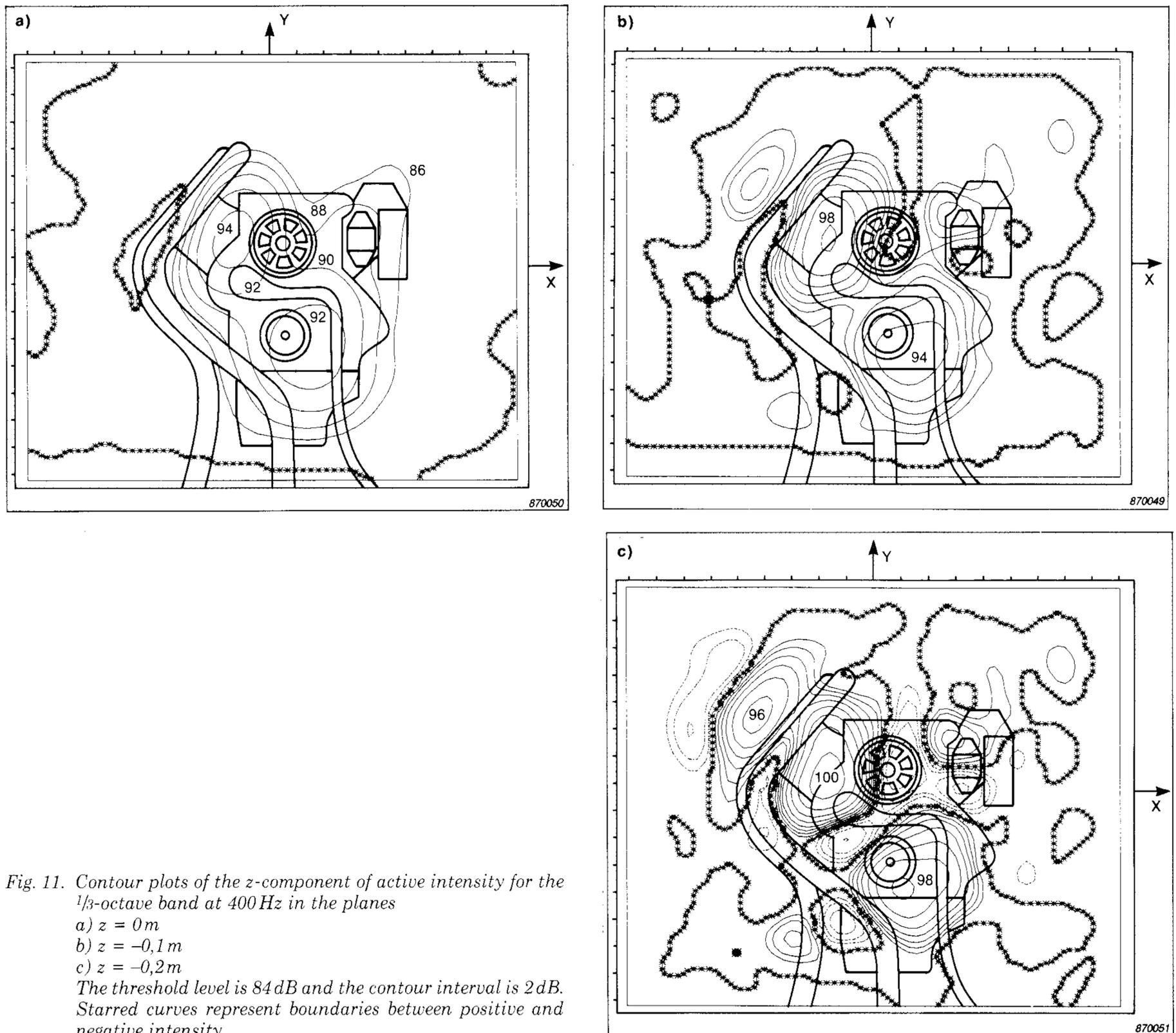
Fig. 11. Contour plots of the z-component of active intensity for the  $1/3$ -octave band at 400 Hz in the planes
