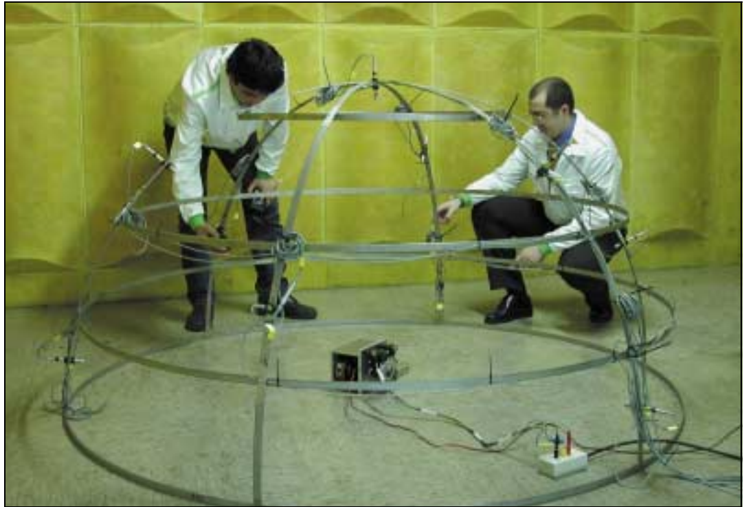
Fig. 1 In an anechoic chamber, the wiper motor under test is placed in a hemispherical frame that holds the array of microphones in position
