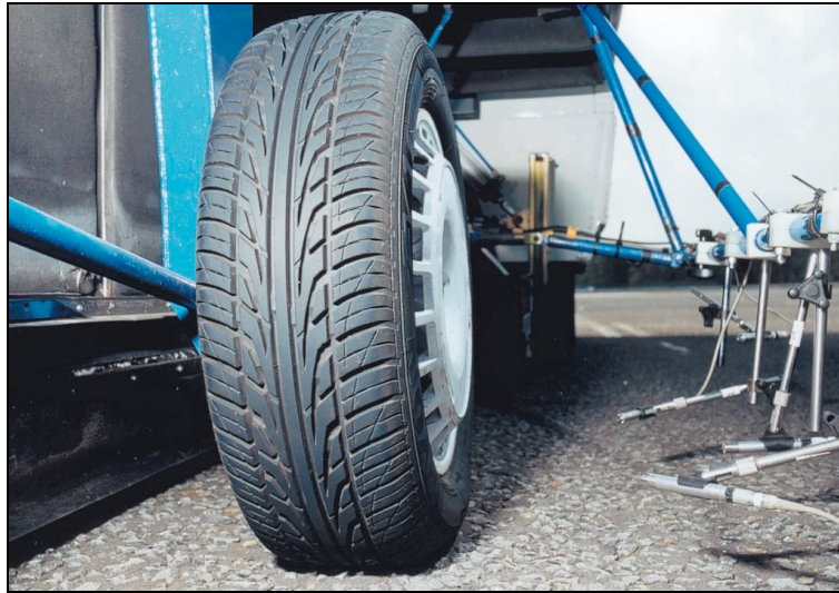
Fig. 2 The test tyre is pneumatically lowered to contact the road surface. The array of seven Brüel & Kjær microphones captures the noise
