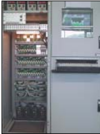
Fig. 4 One of Papst's test control stations at St.Georgen. Every fan is tested electrically and for vibration using a fully automated process
