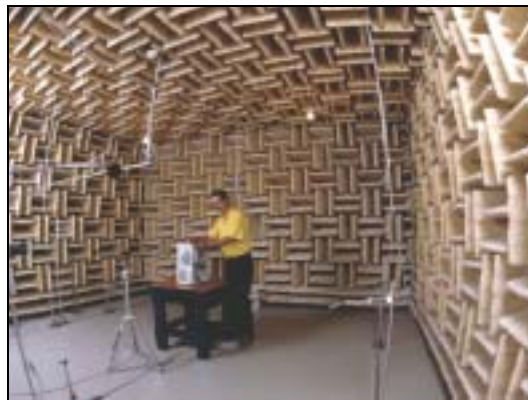
Fig. 3 Papst has a large anechoic room that is completely decoupled from the building and enables very low noise levels to be measured accurately
