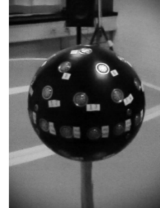
Figure 1: The 52-channel microphone array for HOA used in the current study.
