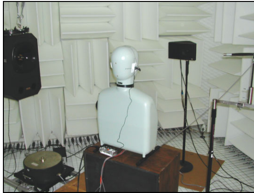
Fig. 5 Inside the R&D lab’s anechoic room, Brüel & Kjær Head and Torso Simulator Type 4128 C evaluates the performance of microphones under various conditions Photo by kind permission of Shure Incorporated
