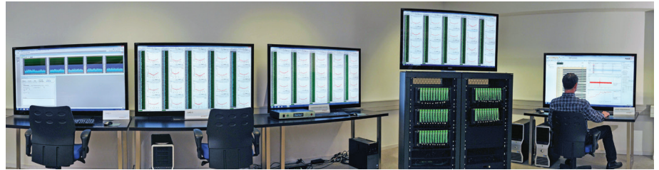
INPE's data acquisition system undergoing testing prior to delivery. The distributed system architecture is shown here collected together, but each workstation is now established in different locations at INPE's facility. At left is the recording control station, the middle three screens show the remote monitoring screens, and right is the post-processing workstation
