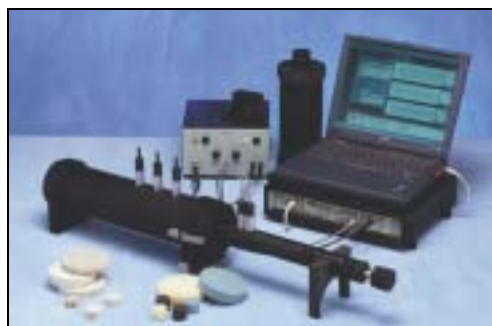
Fig. 3 Material testing (TL measurement) using a Brüel & Kjær Type 7758 PULSE Material Testing System
