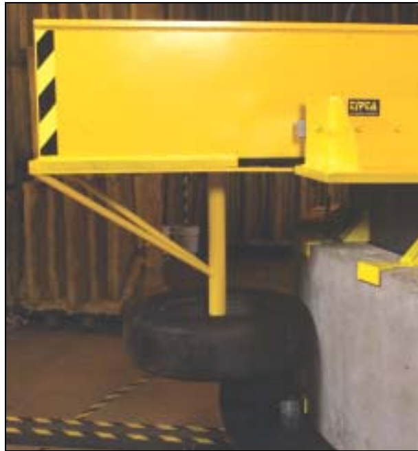
Fig. 4 The tire is in contact with a smooth Portland Cement Concrete (PCC) surface. Screw jacks enable the loading of the tire on the surface to be adjusted at up to 1000 pounds (454 kg)
