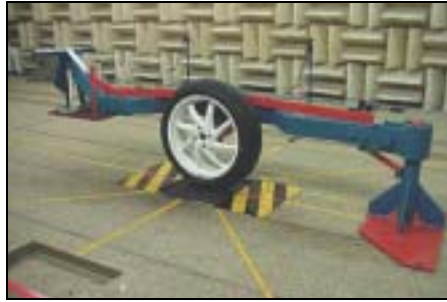
Fig. 5 A specially designed fixture is used to test motorcycle tyres
