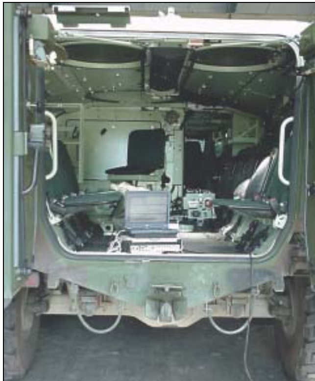
Fig. 2 A Portable PULSE multi-analyzer measures noise and vibration inside a 6- wheeled 25 tonne armoured personnel carrier
