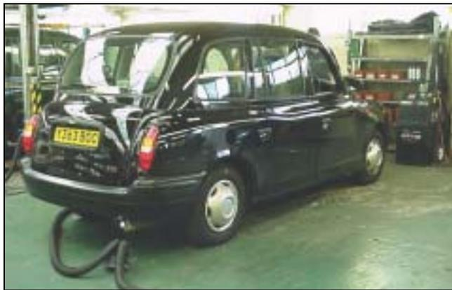
Many sub-suppliers have cooperated with London Taxis International in the development. The TX11 is fitted with the quiet, clean and efficient 2.4 litre Ford Duratorq 90 PS diesel engine with turbo and intercooler. A special steel chassis is manufactured by Thompson Chassis while the manual transmission is from Ford. The automatic transmission is made by Jatco in Japan. LTI produces its own bodies.
