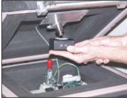
Fig. 5 A Brüel & Kjær Type 4231 Calibrator is attached to the microphone in one of the test boxes
