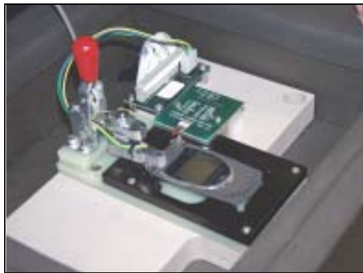
Fig. 6 A mobile phone is placed in the fixture, ready for testing
