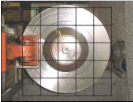
Fig. 2 6 × 6 grid of 36 microphones was used to measure noise from the simple test brake
