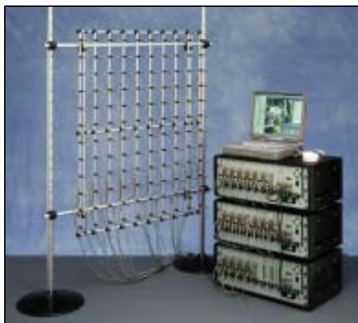
Fig. 1 Three PULSE Type 3560E frames were stacked together to provide up to 132 channels. This array uses 120 microphones
