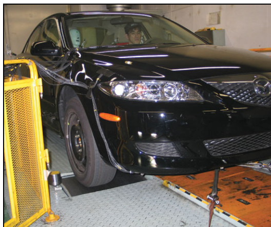
Fig. 3 The 220-channel PULSE-based OMA system is also used on the chassis dynamometer test bench in order to investigate the vibration characteristics of the powertrain
