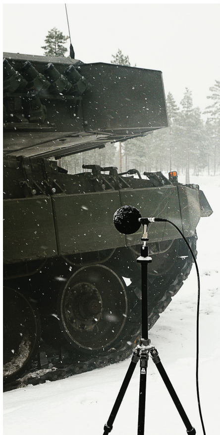
A Type 4189 microphone records the sound pressure levels of a 60-tonne Leopard 2 battle tank
