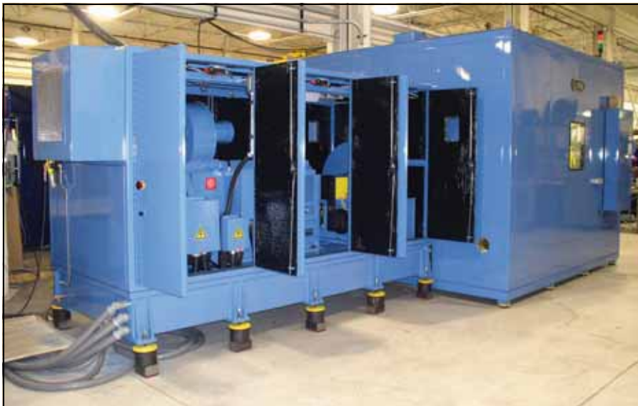
Link Engineering's Model 3900 Brake Noise Dynamometer
