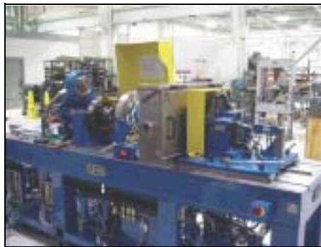
Fig. 8 This dynamometer tests the properties of materials used in aircraft braking systems
