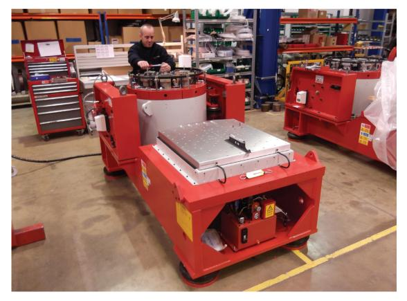
A shaker on the Royston production line in the final stages of assembly
