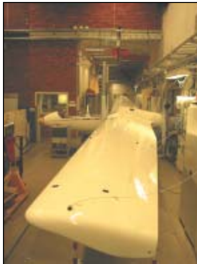
Fig. 5 Experimental structural dynamics – modal analysis is made on the structure of a glider. In the foreground, note the accelerometer fixed to the end of the wing
