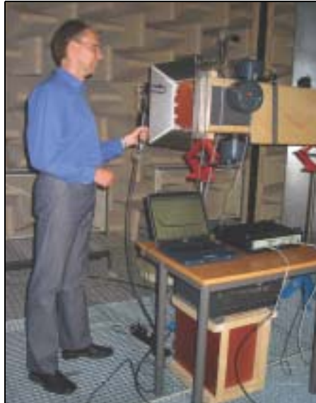
Fig. 10 Senior researcher Per-Olof Berglund makes measurements in the anechoic room using PULSE and a sound intensity probe
