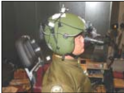
Fig. 7 Tests are made under a variety of conditions. These include the wearing of night vision equipment. A triaxial accelerometer is placed on the top of the pilot's helmet
