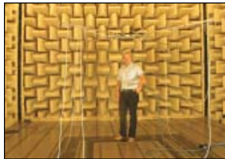
Fig. 3 Measurement of sound power on a handheld pneumatic tool in the semi-anechoic chamber
