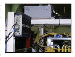
Accelerometers Type 4514-B located near each motor and in the middle of each side rail. These measure the vibration from the DC motors. In addition to the vibration measurement, a current probe clamp is also installed over the power lead to the sunroof, and the signal used to determine the RPM of the motor. The test takes about one minute. On average, the throughput is one complete sunroof system every three minutes on each production line.
