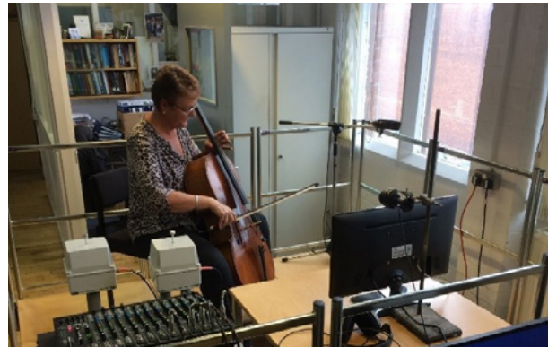
Cellist using a pickup to convert the sound of a cello into vibration which can be felt through the shakers
