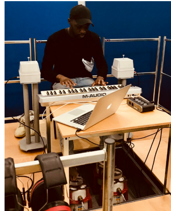
SignKid using four vibrotactile foot shakers to jam in time with a multitrack recording
