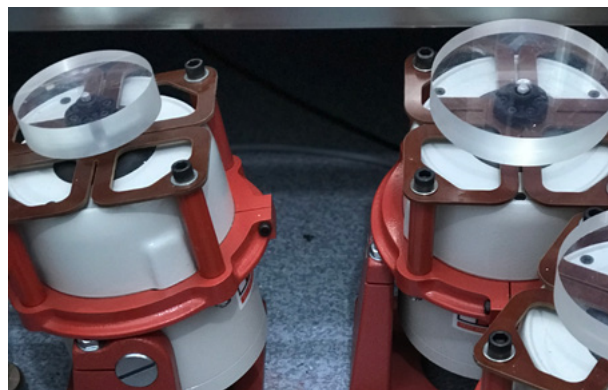
Left: The contactors to the skin were Perspex discs screwed into the shakers with diameters of 2 cm, 12 cm and 10 cm for the fingertip, forefoot and heel respectively; Right: Checking the vibration output using a hand-held vibration indicator.
