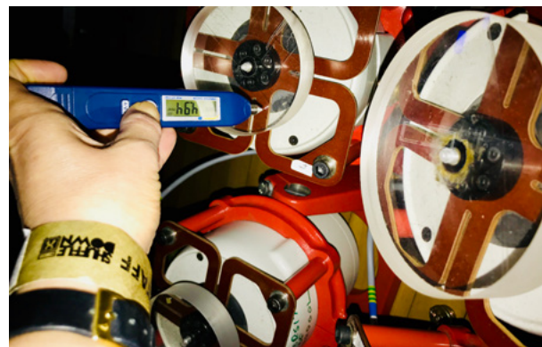
Left: The contactors to the skin were Perspex discs screwed into the shakers with diameters of 2 cm, 12 cm and 10 cm for the fingertip, forefoot and heel respectively; Right: Checking the vibration output using a hand-held vibration indicator.
