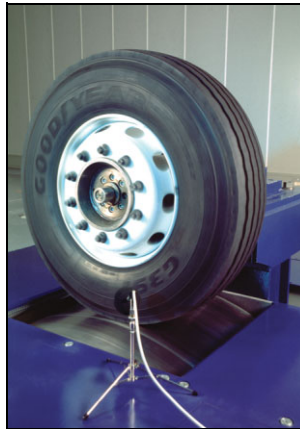
Fig. 6 Truck noise test using a PULSE system
