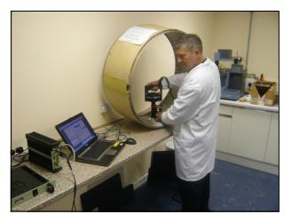
GKN has carried out pure tone tests at a user-specified frequency and broadband noise tests, up to 155 dB overall sound pressure level, measured at the face-sheet. on small scale, flat acoustic material specimens, as well as full scale panels. This is within a design down selection exercise, whereby a comparative analysis of these measurements with the prediction of a proprietary normal impedance prediction model, has also been performed.
