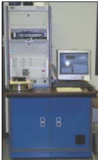
Fig. 6 Each of the four brake testing dynamometers has its own Link Engineering control station
