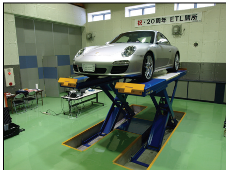
Test preparatory room with car lift
