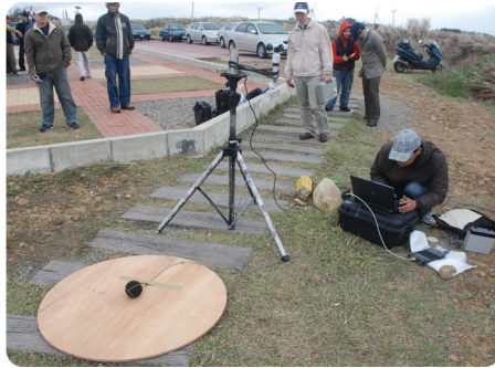
Fig. 2 Making measurements at Miaoli County Chunan Tawn wind farm. The microphone is mounted at the centre of a flat board with its axis pointing towards the wind turbine
