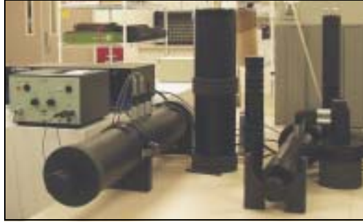
Fig. 3 A Brüel & Kjær PULSE Material Testing system Type 7758 is used in Dow's laboratory to test the acoustical properties of materials
