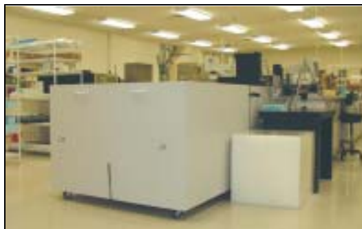
Fig. 4 Dan Schroer has designed a built a special transmission loss test setup. The chamber is shown in the foreground
