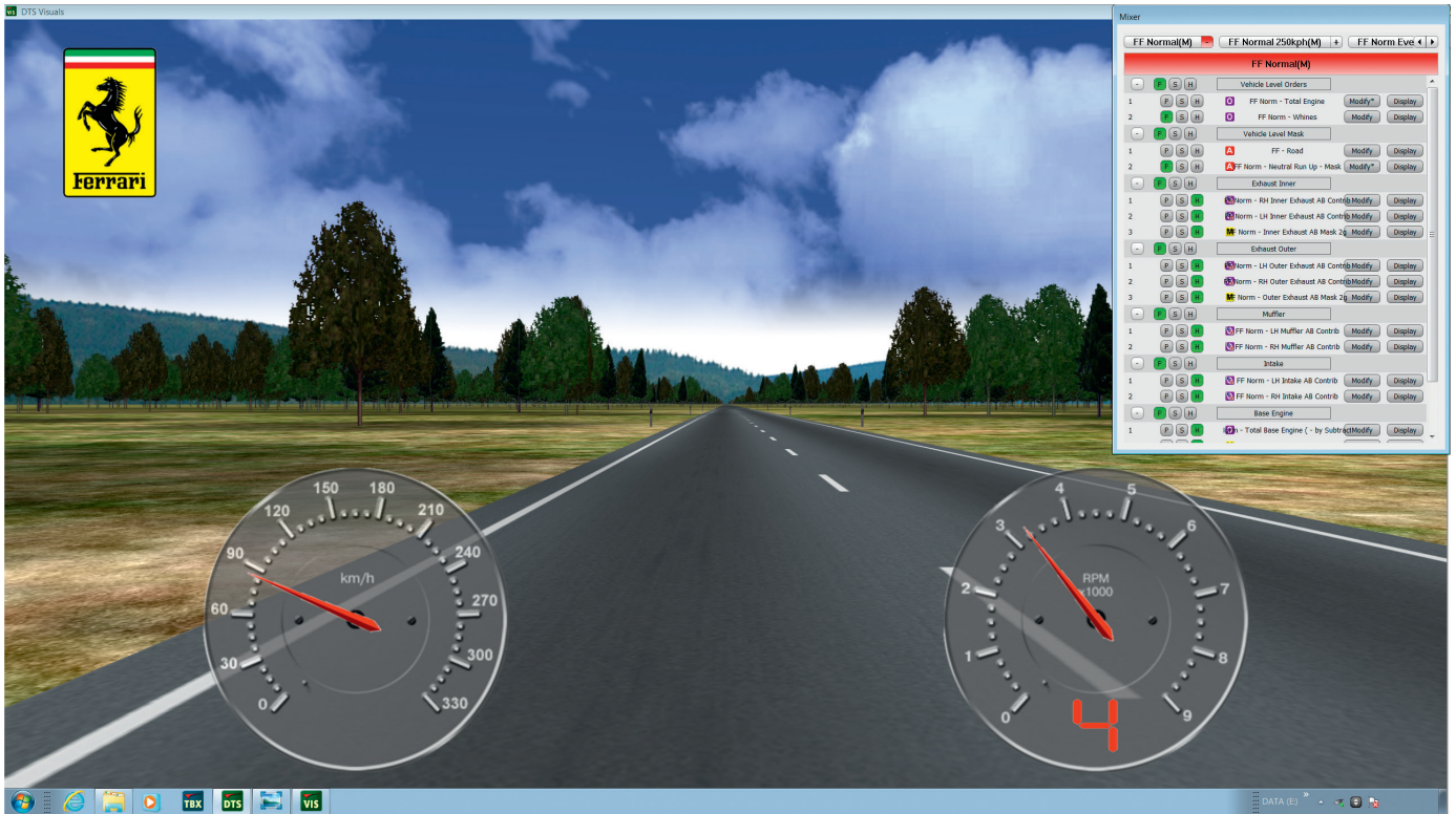
Brüel & Kjær's Desktop NVH Simulator enables Ferrari to evaluate, modify and design NVH data interactively, by driving in a virtual scenario using authentic car controls and feedback. The scenario, shown on desktop monitors, allows quick changes between different vehicles, systems and components.
