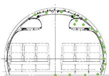
Distribution of multi-field microphones in the cavities between the cabin and the fuselage
