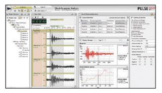
The aim of the SRS calculation is to convert motion input to a set of single degree of freedom (SDOF) damped oscillator responses calculated in the time domain. The response amplitudes of the oscillators are plotted as a function of SDOF frequency to produce the shock response spectrum.
