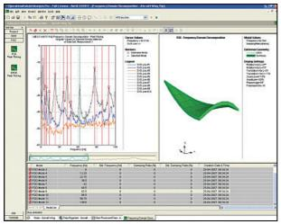
PULSE Operational Modal Analysis Type 7760 is an analysis tool for effective modal identification in cases where only the output is known. The software allows you to perform accurate modal identification under operational conditions and in situations where the structure is impossible or difficult to excite using externally applied forces.
