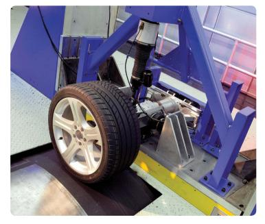
Each test takes about two minutes, and then an average of a number of tyre rotations is taken. The intention is to evaluate peaks in the range from zero to 6.4 kHz, and specifically, the engineers are interested in four ranges between 4 and 260 Hz – which are in the range where tyre rumble is found.
