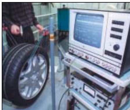
Fig. 2 One method of performing modal analysis on tyres. The tyre, mounted on a rim, is suspended on rubber shock cord. The tyre is excited by an impact hammer and the response is measured by an accelerometer
