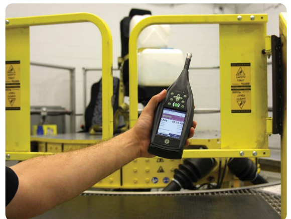
Type 2270 at work checking the sound level of their six-axis MTS system. According to Logan Mullnix, "It is a valuable tool for benchmarking and troubleshooting industrial-type noise problems, easily providing overall levels and 1/3 octave spectra."
