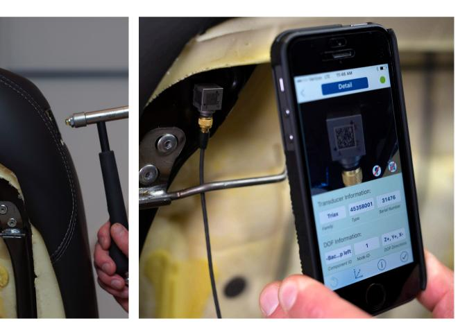
transducer and trace its cabling through to the data acquisition hardware, before they can manually add information about its alignment and location.
