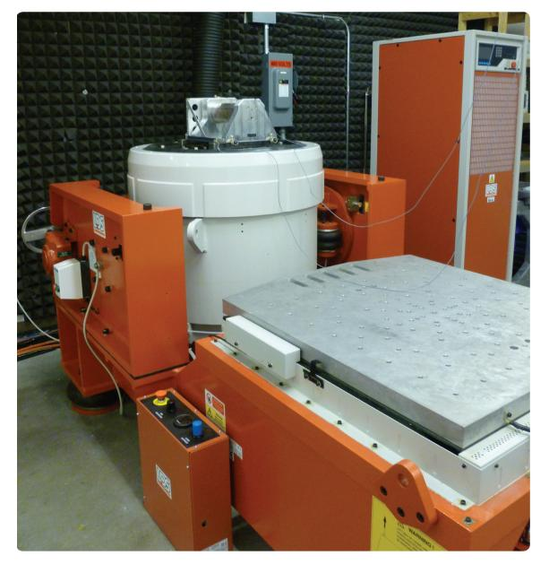
**Sinusoidal** tests are used for propeller aircraft applications, to simulate windmilling (an imbalanced engine while in flight), and tyre bursts.
