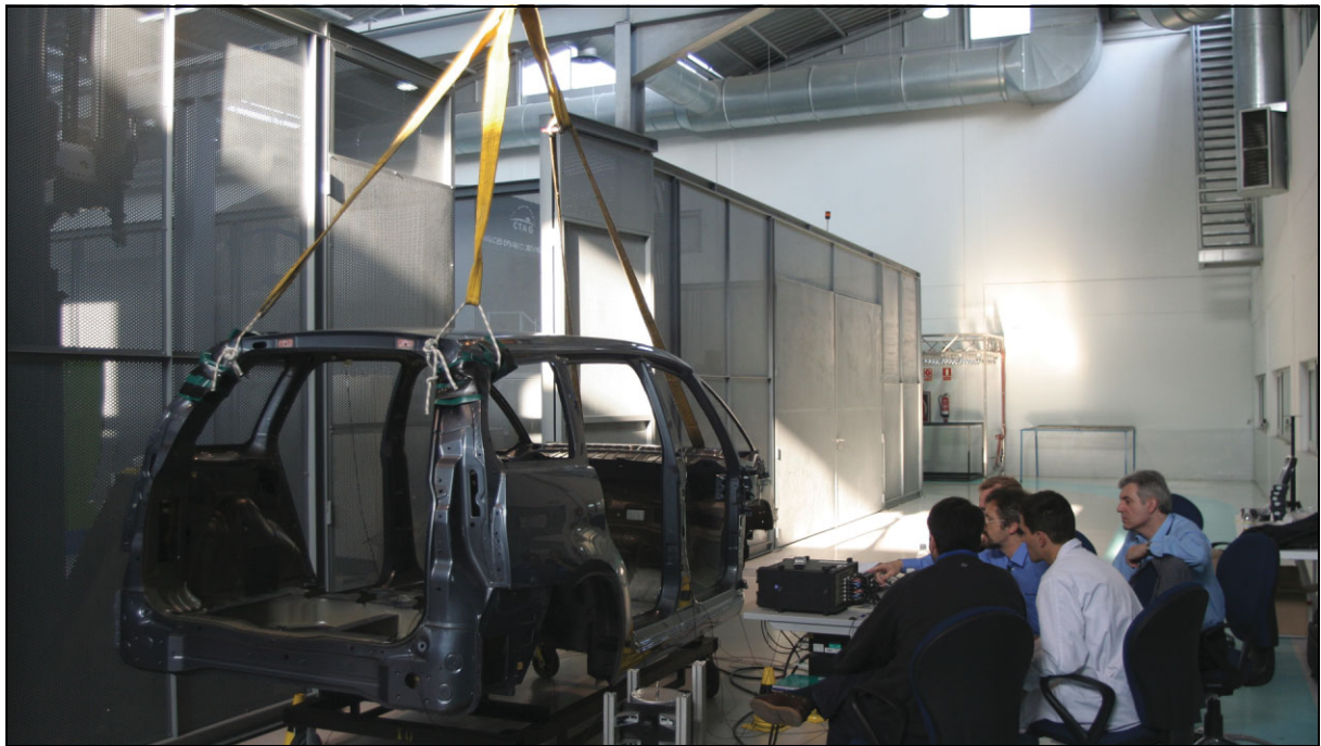
Fig. 1 BIW (Body-In-White) modal testing of a Citroën Picasso C4 using MIMO (Multiple Input Multiple Output) analysis
